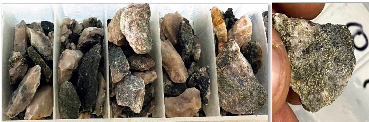
Drill hole HWRC039; chip tray record showing drill chips from 23-28m that intersected a sulphide-rich carbothermal unit. The interval shown returned an assay of 5m @ 9.73 g/t Au, 10,154 WO 3 (results for other metals awaited).
