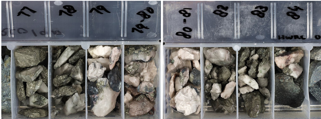
Figure 2. Drill chips from RC drill hole HWRC0198 (76-84m) – sulphide-rich carbothermal zone.
