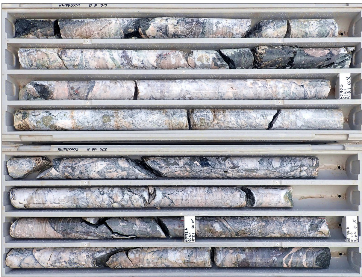
Figure 5. Example of solid drill core from diamond hole HWDD0005, highlighting part of a 10m wide sulphide-bearing, carbothermal zone (~88.6 to ~95.5m shown).
