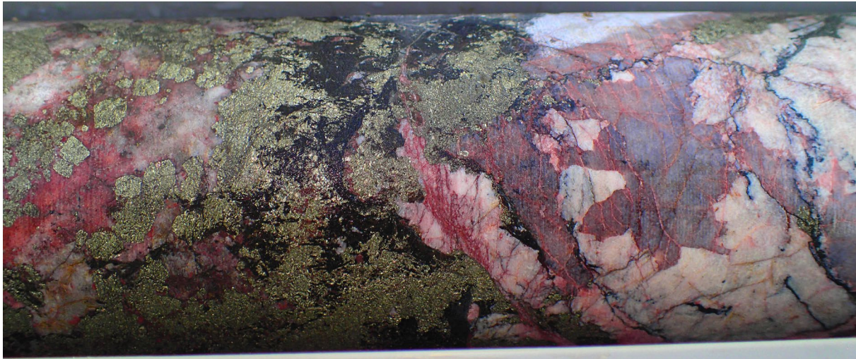
Figure 4. Example of solid drill core from diamond hole HWDD0002, showing close-up example of a spectacular, sulphide-rich carbothermal unit at a depth of 83m.
