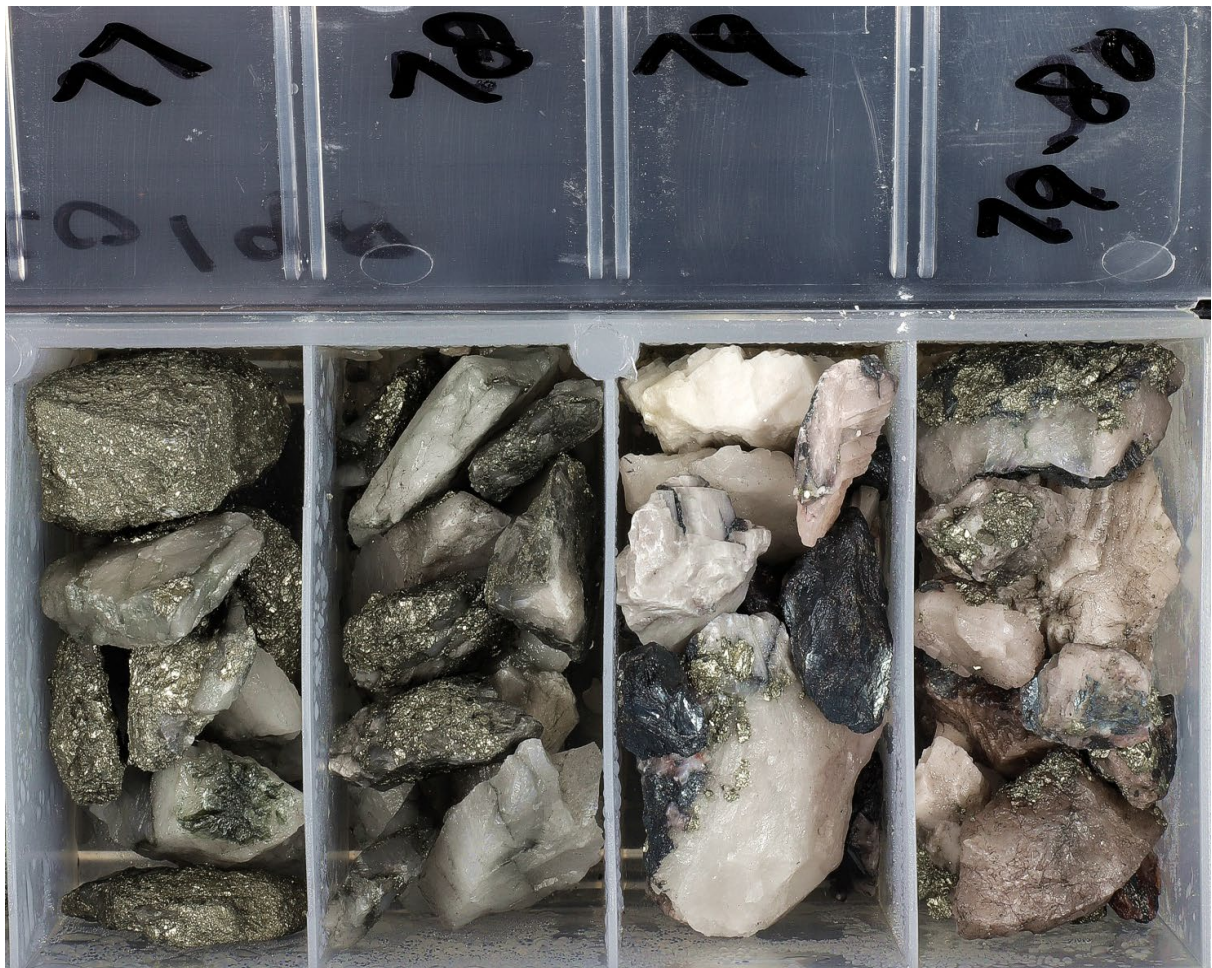
Figure 3. Close-up of drill chips from RC drill hole HWRC0198 (76-80m) – sulphide-rich carbothermal zone.
