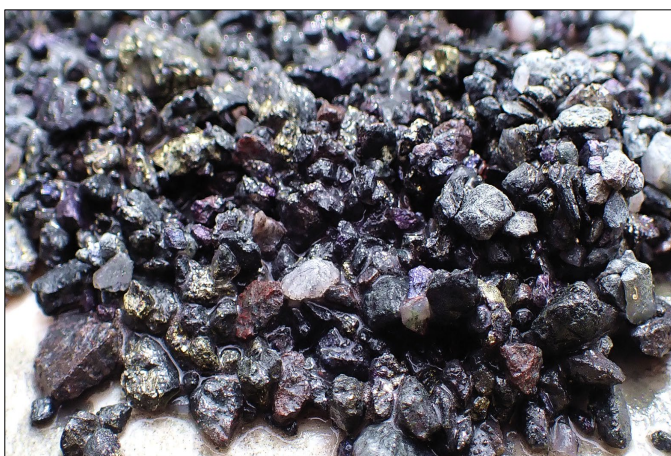
Example of RC drill chips with copper sulphide chalcopyrite (yellow), and high-grade copper sulphides bornite (purple) and covellite (blue), in quartz breccia. This sample from a depth of 125m in drill hole MERC0017, returned an assay of 17.5% copper.
