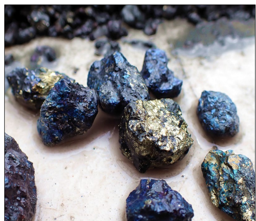
Example of RC drill chips with copper sulphide chalcopyrite (yellow), and high-grade copper sulphides bornite (purple) and covellite (blue), in quartz breccia. This sample from a depth of 125m in drill hole MERC0017, returned an assay of 17.5% copper.
