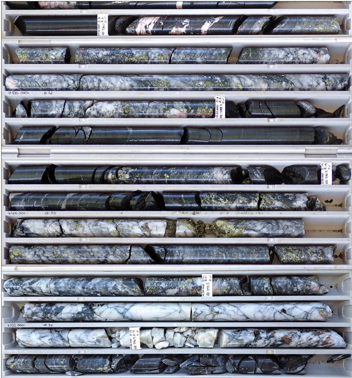
Diamond core drill hole HSDD0001 that intersected a 10-metre zone of high-grade copper sulphides (chalcopyrite) at the Horseshoe prospect, from 285 metres. Assays pending.
