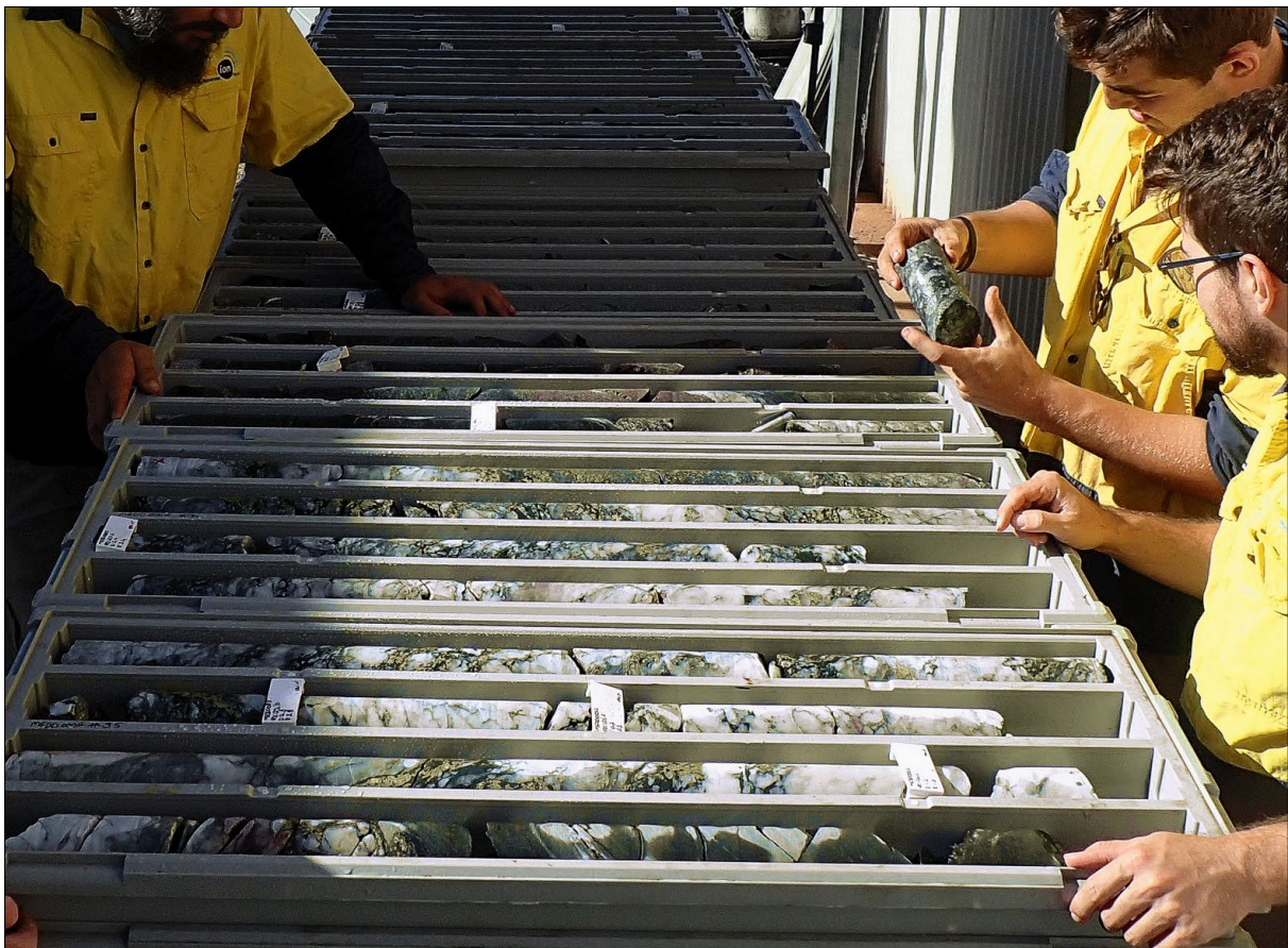
Excited geologists inspect diamond core drill hole MEDD0002, that intersected a 10-metre zone of high-grade copper sulphides from 117 metres at the Meteor prospect. Assays pending.
