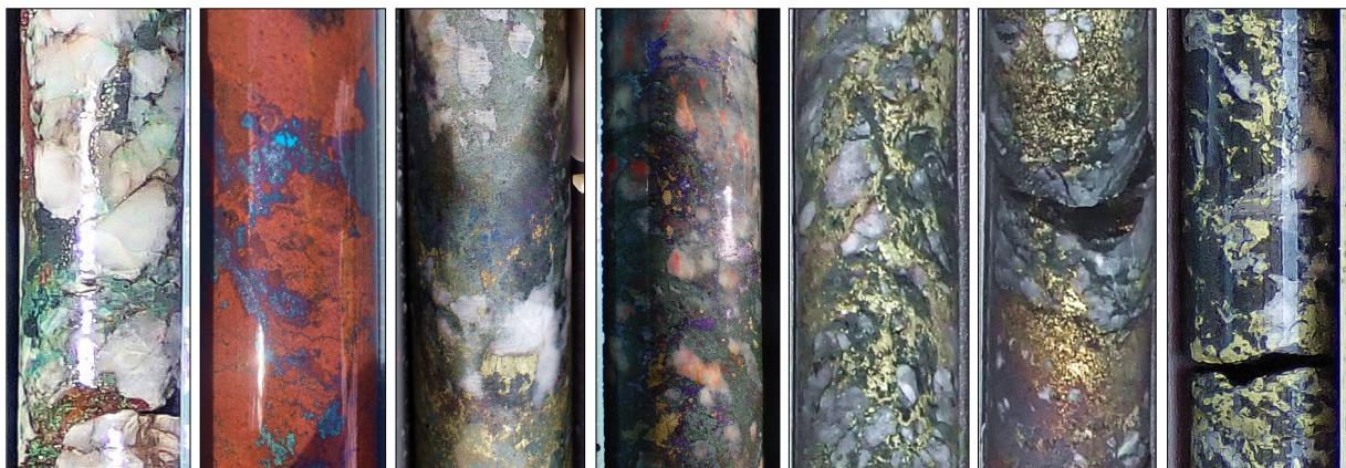
Figure 3. Diamond drill core showing examples of copper mineralisation at New Dollar, Meteor and Horseshoe.
